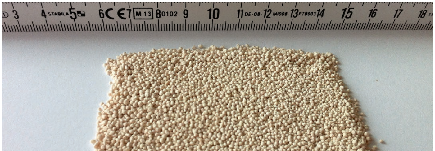
Fig. 2: Extra fine granulometry of Easy Start®
